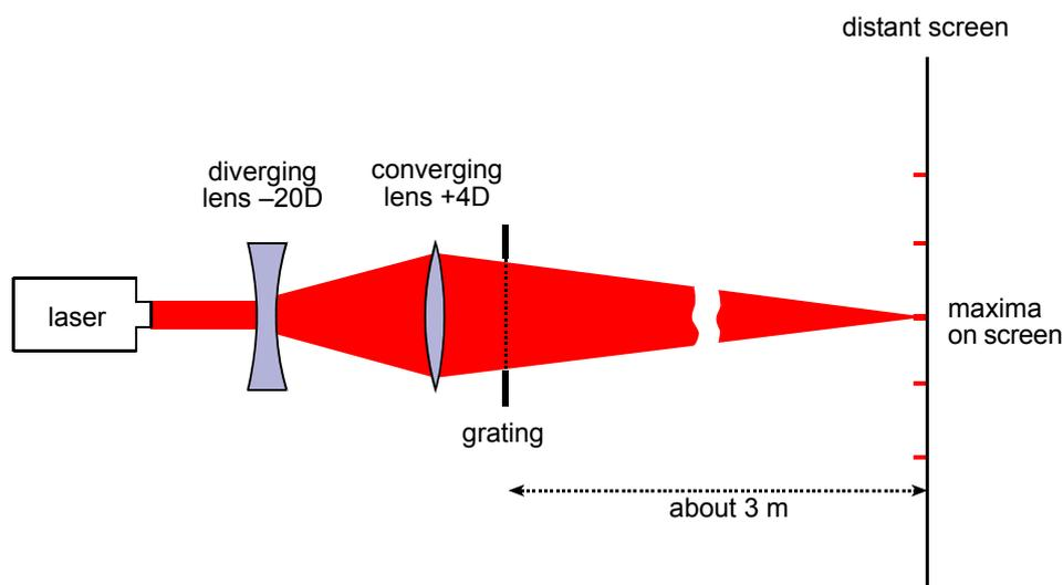
The idea is to shine the laser light through a grating – an array of many slits, not just two. To get the laser beam to go through many slits it has to be broadened. That is what the lenses in the diagram are for.
