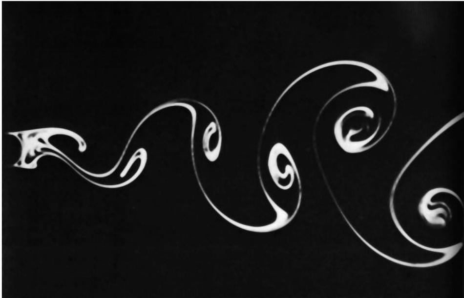
The vortices generate alternating high and low-pressure regions on the downwind side of the body, in this case the bridge. Such vortices are called Strouhal vortices and are shed at a rate determined by the equation
