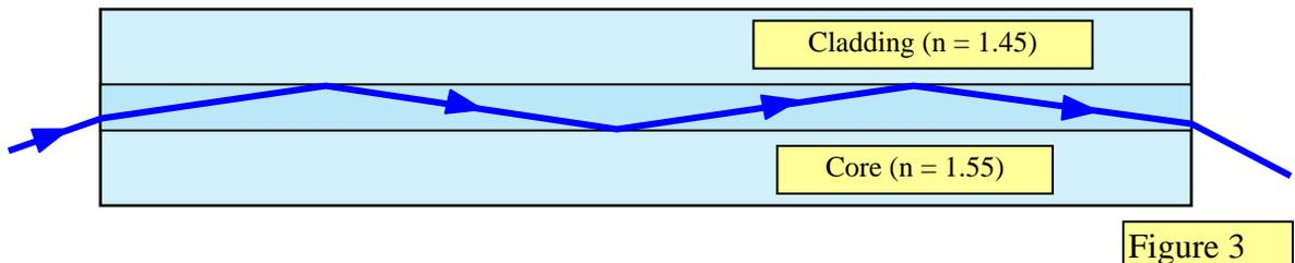
The cladding increases the critical angle between the two materials. The benefits of this are:
