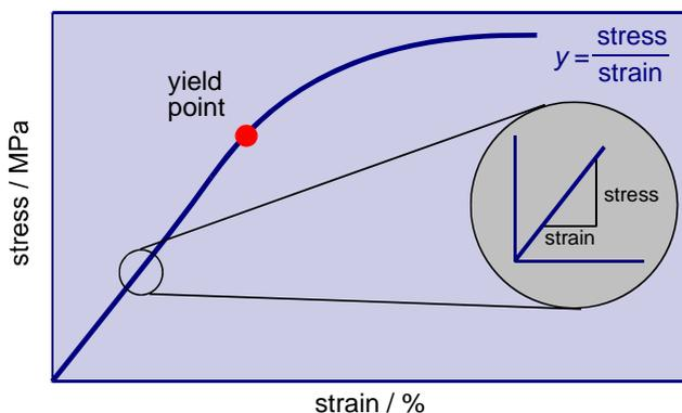
The initial straight-line part of the graph shows that the strain is proportional to the stress.
