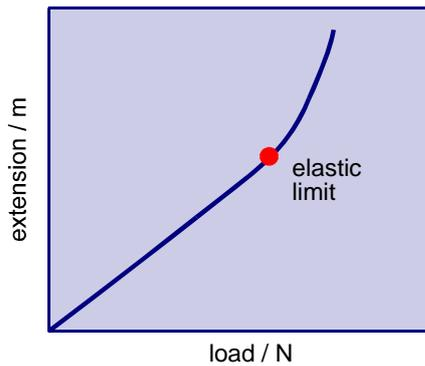
A graph is a good way to show this behaviour, one way is above, but it's usual to plot load on the y-axis and extension on the x-axis so that the spring constant  $k$  is measured in  $\text{Nm}^{-1}$  is the slope of the graph. (For the reason see: TAP 227-2: Tension and extension)
