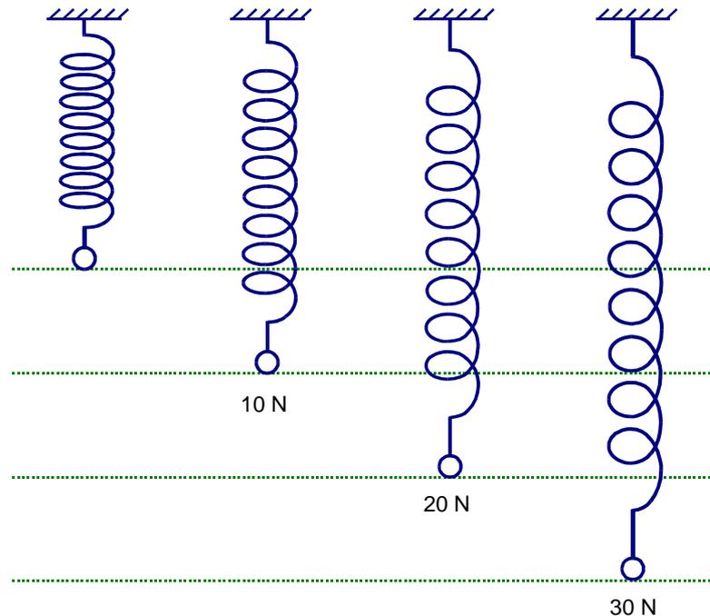
You have probably done an experiment like the one shown here; use a load to stretch a spring, and the increase in length (extension) of the spring is proportional to the load. If a spring (or anything else) behaves like this, with extension proportional to load, we say that it obeys Hooke's law.
