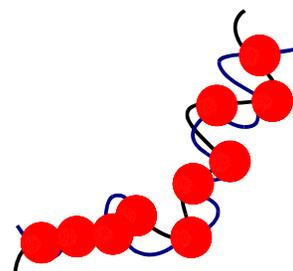
Bakelite has massively cross-linked chains. The cross-links stop the chains from unfolding.
