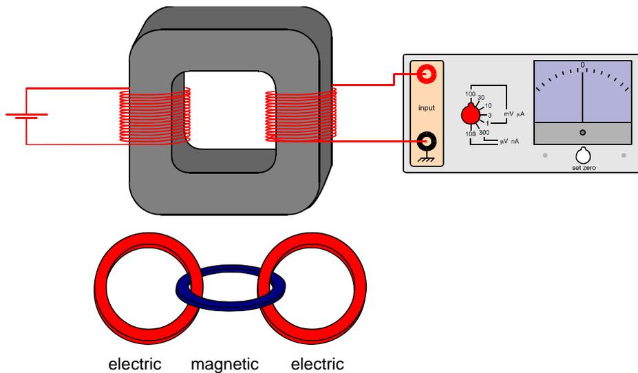
The interlocking electric and magnetic circuits are quite crucial to the operation of electromagnetic machines such as transformers. A break in the primary electric circuit leads to a change in the magnetic circuit and correspondingly induces an emf in the secondary electric circuit.
