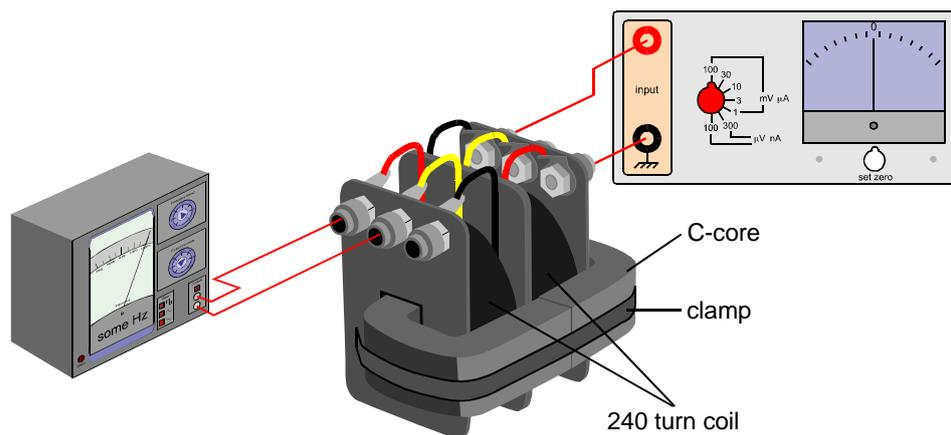
1. Set the signal generator to produce a square wave oscillating below 1 Hz. This is just like the previous experiment, switching the current on and off.
