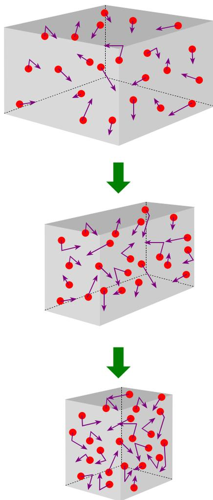
You need to measure how the volume of a fixed number of particles affects the pressure. Squeezing these particles into a smaller and smaller volume results in more and more
