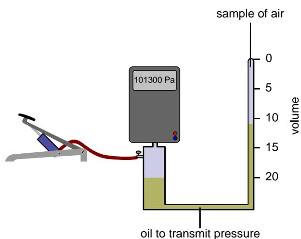
1. Take readings of pressure and volume for a suitable range of volumes, determined after a pre-test. Plot a graph as you go.
