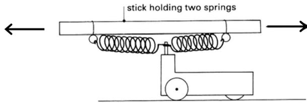
Mechanical analogue of an  $LC$  circuit.
