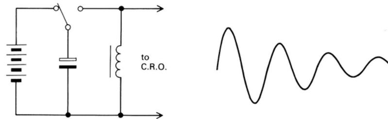
The cells are used to charge the capacitor which is then discharged through the inductor. With the time-base set to a slow speed, decaying oscillations can be observed. Changing the capacitance (or the inductance) will alter the frequency.
