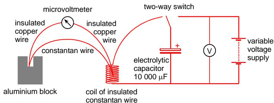
Make sure that the capacitor is connected to the supply correctly otherwise it may suffer damage. You will need to use the thermocouple connected to a sensitive voltmeter, measuring in mV.
