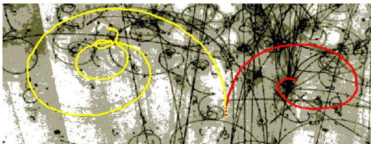
In this case the chamber is filled with liquid hydrogen mixed with liquid neon. It is held under pressure which is released just as the particles enter the chamber to encourage bubbles to form and enlarge near the ions.
