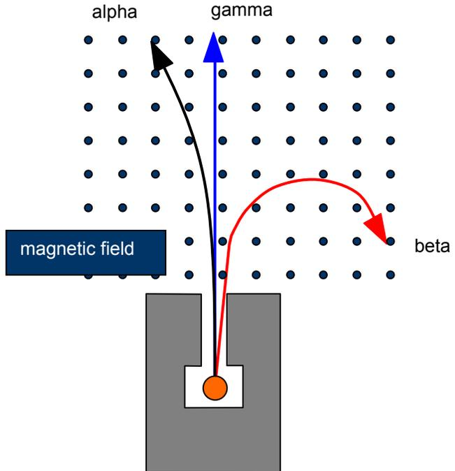
**NB** The diagram above is common in textbooks, but is ONLY illustrative. For the curvature shown of beta particles, the curvature of the alpha tracks would be immeasurably small.
