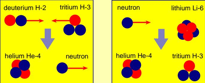
Deuterium and tritium are heated to very high temperature. Neutrons from their fusion then fuse with lithium in a 'blanket' around the hot gases. Tritium is renewed.
