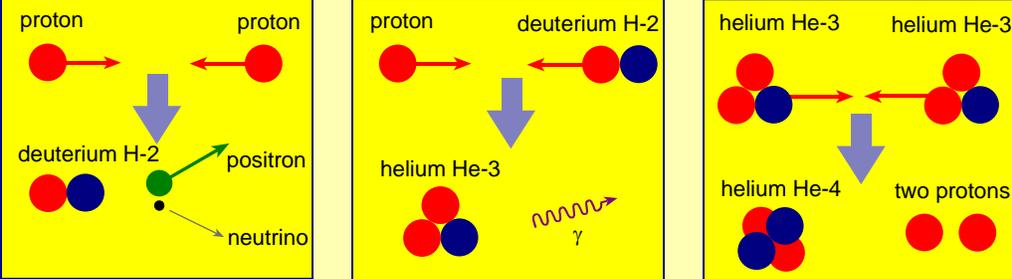
Two protons fuse, converting one to a neutron, to form deuterium H-2.
