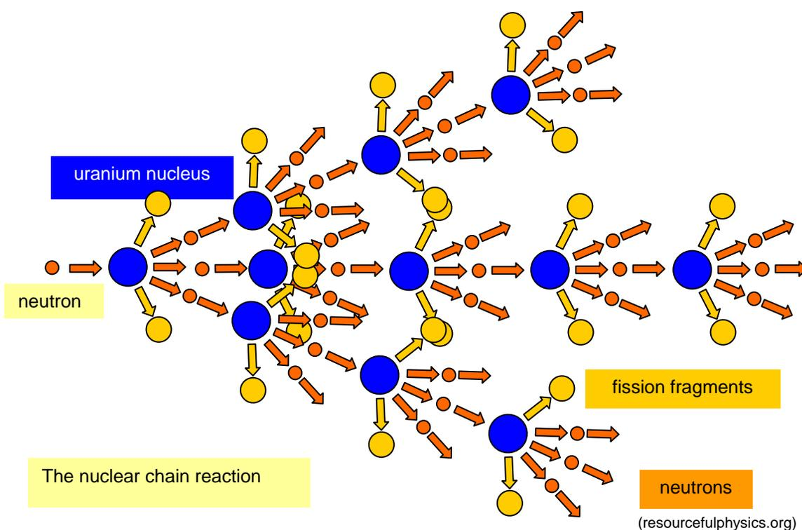
mutual coulomb repulsion between the two ends drives the fission process. An alternative is to grease a plate and put a large drop of water on it. Wobble the plate about and watch the drop split.
