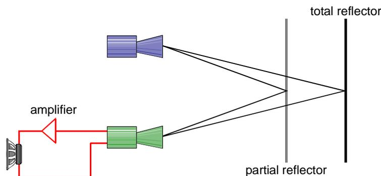
If necessary, set the transmitter to unmodulated microwaves. Put the hardboard sheet near the transmitter and receiver. Make sure that you have room to swing the metal sheet and then move it as fast as possible away from the hardboard.
